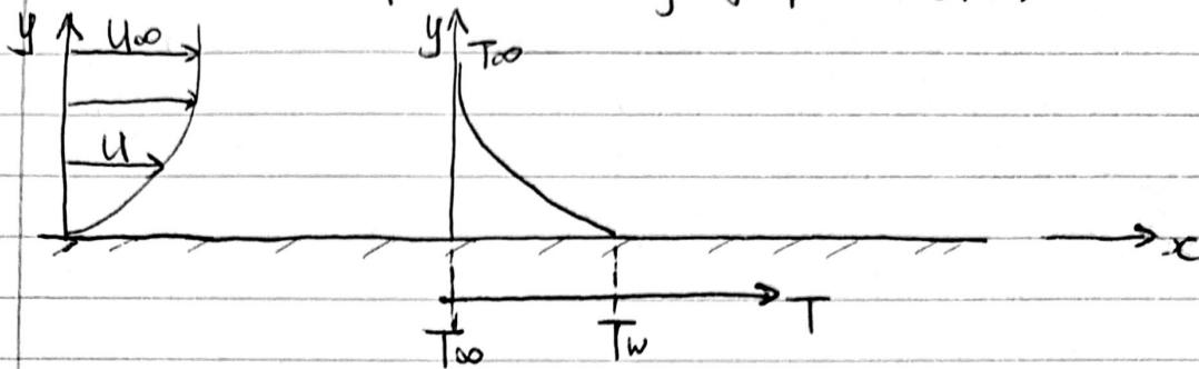
The heat exchange between the wall and the fluid can be expressed as the heat conducted away from the wall by the fluid (Fourier's Law)
