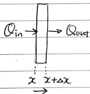
$$\Delta x \dot{q} + Q_{in} - Q_{out} = \text{energy gain}$$
